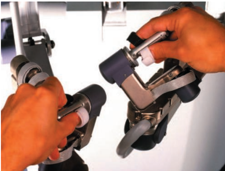
FIGURE 2 EndoWrist® instruments are controlled from a remote surgical console. the current flows through a conducting cable to an active or positive electrode, which contacts the patient tissues at the point of desired effect. The current passes through the tissue and returns back to the generator via the patient's inactive or return electrode. In monopolar ESU, the flow of electricity occurs in one direction, in that, the active and inactive electrodes are separated by a significant distance, resulting in the need for the electrical energy to pass through adjacent body tissues before contacting the return electrode. As electrical current will follow the path of least resistance in returning to a ground, this current pathway may inadvertently include tissues that can be damaged by this flow
