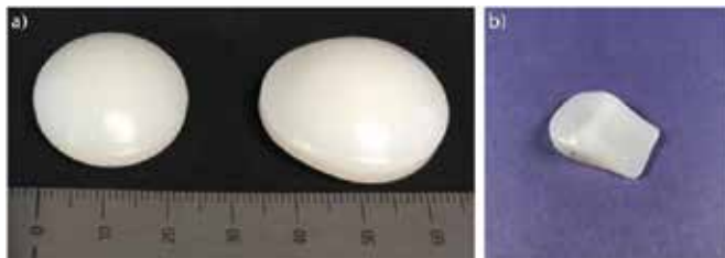
Fig. 1 The patellar component comes in various shapes: (a) shows a symmetric (left) and asymmetric (right) patellar component which attempts to better reflect the naturally occurring asymmetric shape of the patella; (b) shows a different asymmetric component design.
