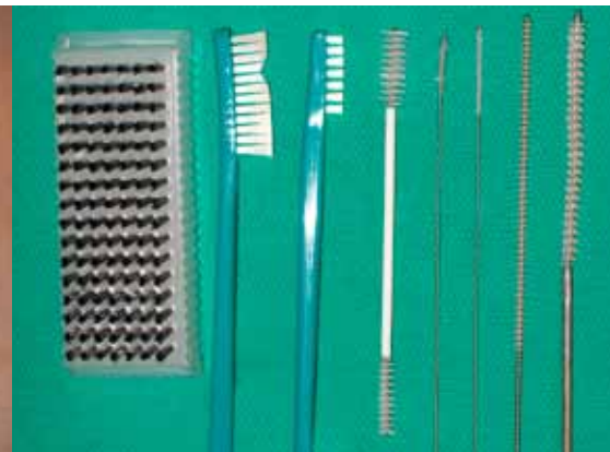
A sampling of brushes used in the decontamination area of sterile processing. Some brushes, like the slender ones, are designed specifically for cleaning lumens
